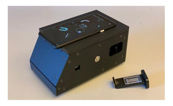
A photo of a device attached to an ordinary smartphone that can detect the presence of SARS-CoV-2 in a nasal swab. Credit: Daniel Fletcher and Melanie Ott
