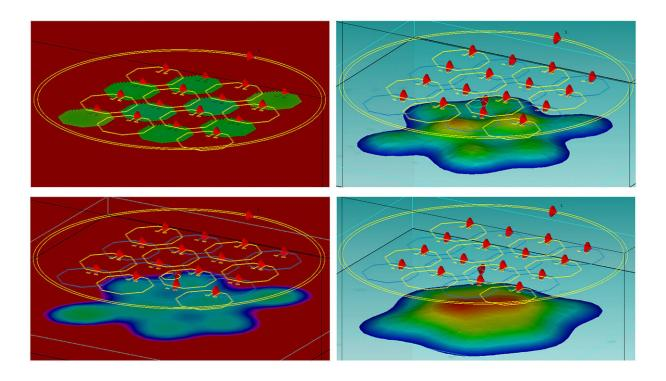
Phase images at two different depths (left) and magnitude images of the magnetic field (right) for different resonance patterns in a metamaterial array. Credit: Fraunhofer MEVIS
