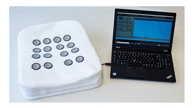
In a total of 16 channels, the recording device developed at TU Graz records the lung sounds during breathing. Credit: TU Graz
