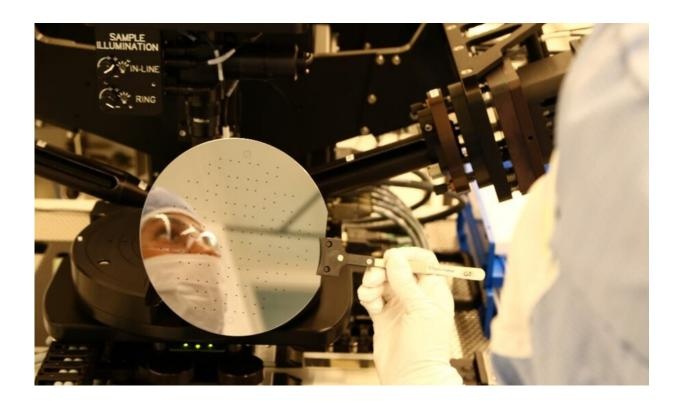
Researcher and author Elizaveta Vereshchagina in the laboratory. Microfluidics technology has a variety of applications, including DNA analysis and organ-on-achip. The photo shows a 6-inch silicon wafer during processing in cleanroom. The dots are inlets to and outlets from the microfluidic channel. Credit: Norwegian University of Science and Technology
