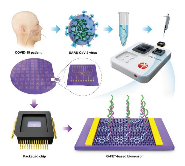
Top left: Extraction of viral RNA. Bottom left: From Si wafer to plug-and-play graphene packaged chips. Top right: Home-developed portable electrical detector. Bottom right: Illustration of the ss-DNA probe immobilization onto graphene using a typical PBASE linker, followed by hybridization with an RNA
