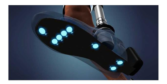
Signals from tactile sensors under the sole of the prosthetic foot and from angle sensors in the electronic prosthetic knee joint are passed on to the nervous system. Credit: ETH Zurich
