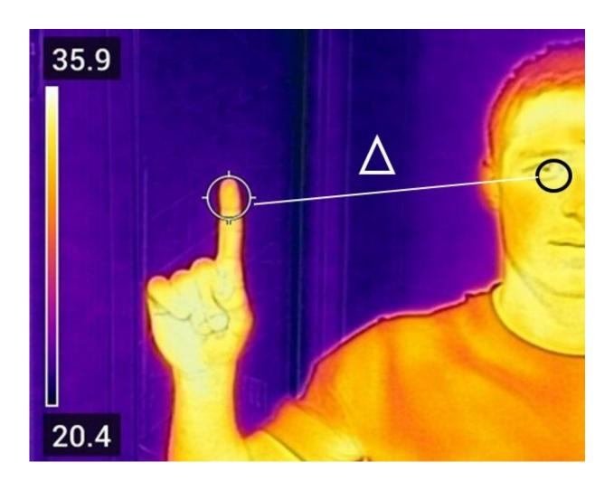
Example of skin temperatures from an IR thermogram. This image was taken in the evening at an ambient temperature of 19°C. Body temperatures at the time were: Core 37.4oC; forehead 35oC; eye 35.6oC; nose 33.8oC; finger 33.3°C. Identifying fever-induced changes in deep body tissue might be improved by including hands in the thermogram and examining the difference finger and eye
