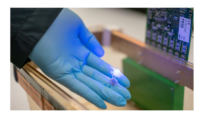
Dr. Sung II Park's paddle-shaped device consists of a harvestor that contains microchips for wireless communication. The harvestor also produces currents to power LEDs inserted near the end of the shaft. Credit: Texas A&M University College of Engineering
