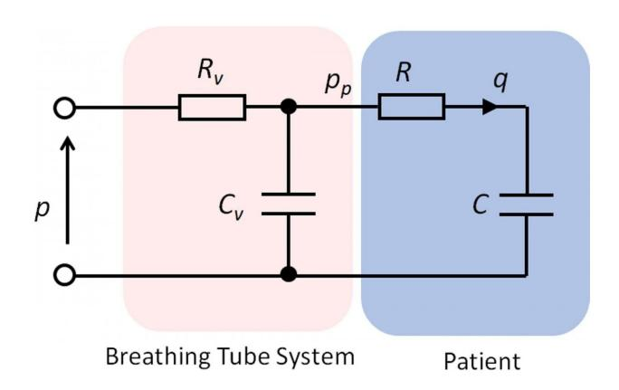
Simple RC network model of ventilator system and patient, with linear resistance (Rv) and compliance (Cv) for the ventilator tubing system, and linear resistance (R) and compliance (C) for the patient. Credit: University of Bath
