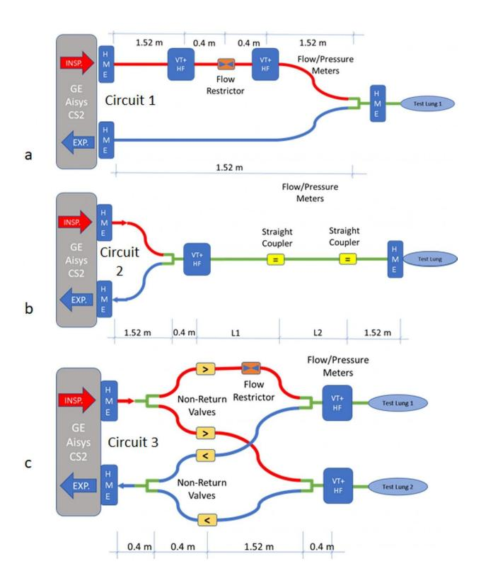
HME = heat and moisture exchanger, VT+ HF = Fluke VT+ HF flow meter, INSP. = inspiration, EXP. = expiration. Credit: University of Bath
