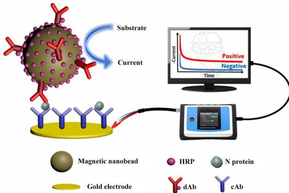
A system developed by Rice University engineers employs a stamp-sized microfluidic chip that measures the concentration of SARS-CoV-2 nucleocapsid protein in blood serum to diagnose COVID-19 in less than an hour. The system uses an off-the-shelf cellphone and potentiostat to deliver the results. Credit: Lillehoj Research Group/Rice University
