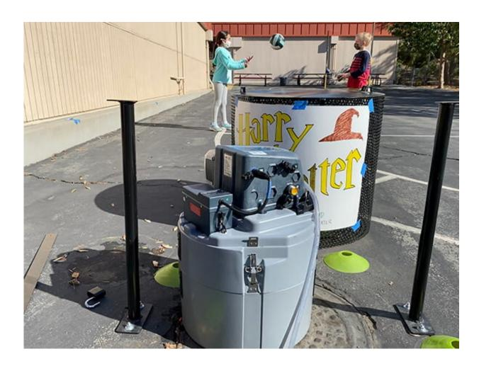
In addition to surface monitoring, a robot takes daily samples of wastewater every 30 minutes to detect the presence of SARS-CoV-2 at each campus. Credit: County of San Diego
