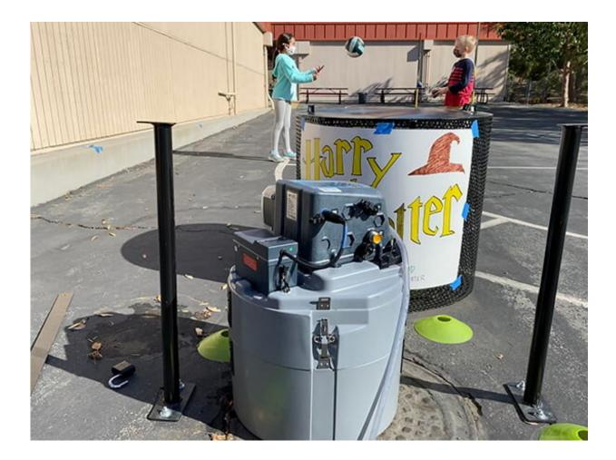
In addition to surface monitoring, a robot takes daily samples of wastewater every 30 minutes to detect the presence of SARS-CoV-2 at each campus. Credit: County of San Diego
