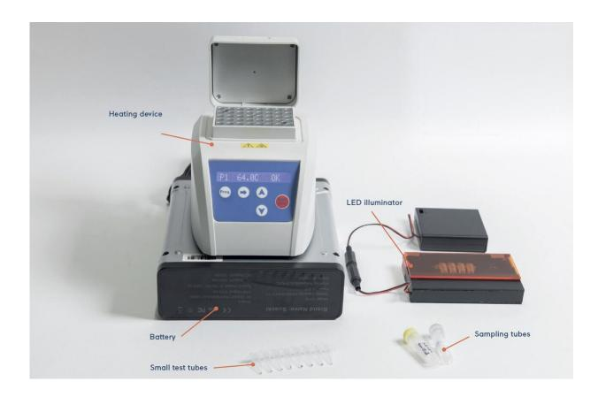
The mobile diagnostic system includes all necessary components — small test tubes, a battery, a heating device and an LED illuminator — and does not require any sophisticated equipment or infrastructure, enabling on-site diagnoses. Credit: Hokkaido University
