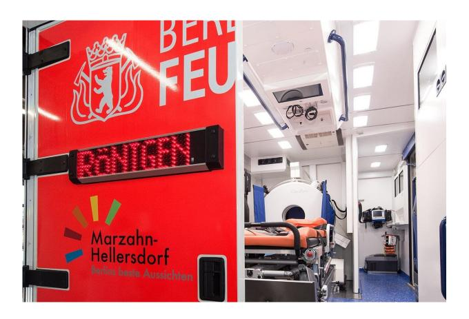
Each STEMO mobile stroke unit is fitted with a CT scanner and a miniature laboratory, enabling the diagnostic evaluation of stroke patients. Credit: Unfallkrankenhaus Berlin (ukb)
