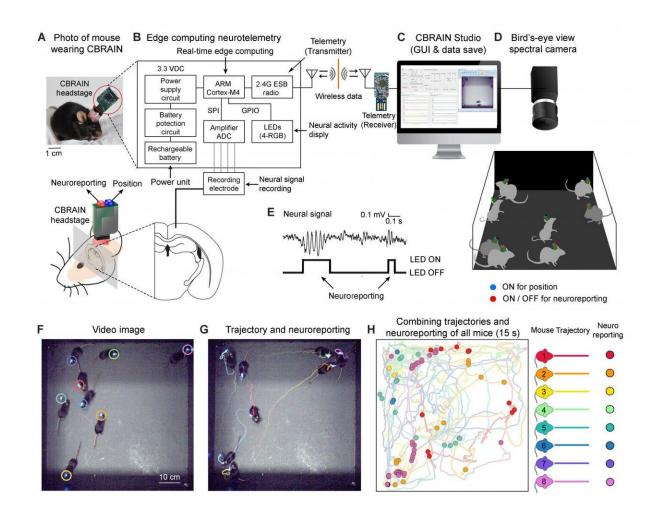
(A to D) Schematic diagrams of the CBRAIN system. (A) Photo of a mouse wearing the 2.6-g-weight CBRAIN headstage. (B) A headstage consisting of an amplifier, edge computing processor, telemetry, and LEDs records, analyzes, transmits BLA signals, and reports the neural activity. A high-speed bird's-eye view spectral camera records the group behaviors and LED lights. (C) The data acquisition software CBRAIN Studio synchronizes and records neural signals
