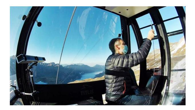
Aerodynamics in the cabin: At the windows, an expert measures airflow using air pressure sensors. Credit: Streamwise GmbH
