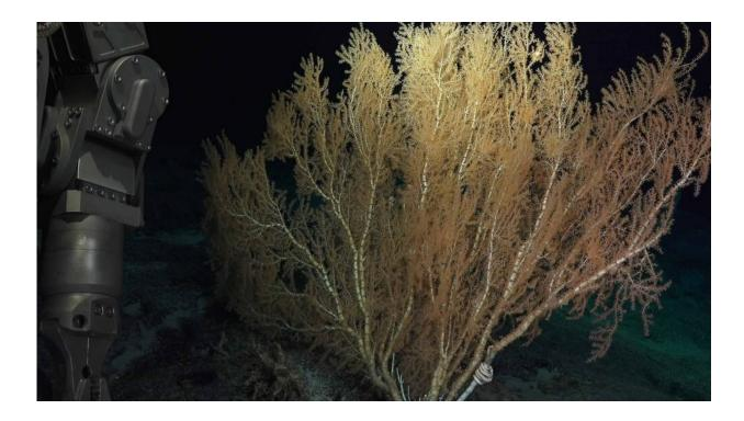
ROV SuBastian setting up to sample a bamboo coral, 2,000 m below the surface, with its robotic arm. Credit: Schmidt Ocean Institute
