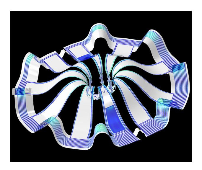
Three dimensional multifunctional neural interfaces for cortical spheroids and engineered assembloids. Credit: Northwestern University
