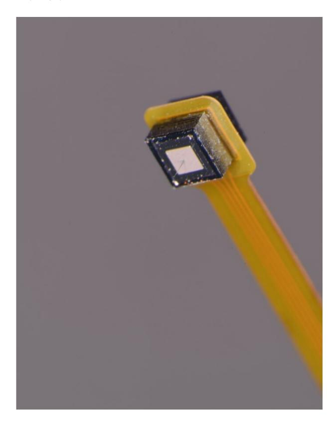
A block module of a 3- $\mu$ m-diameter and 400- $\mu$ m-length needle-electrode
