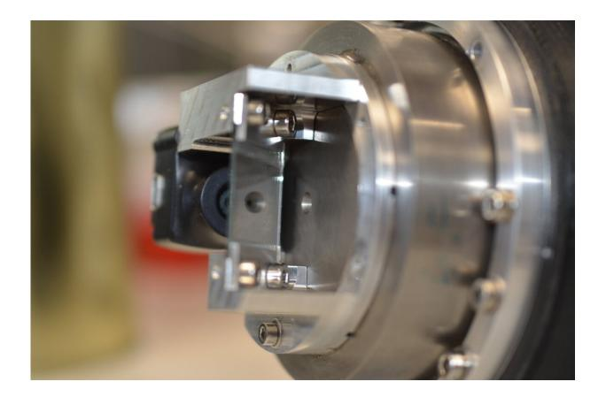
The camera works by using a pinhole in the centre of the device which allows an image of the source of gamma radiation to be taken. Credit: Loughborough University
