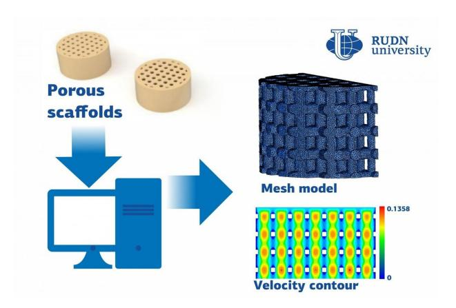
An associate professor from RUDN University found out the effect of the number and size of pores on the permeability of bone implants by biological fluids. The results of the study could help choose the optimal physical parameters of implants. Credit: RUDN University
