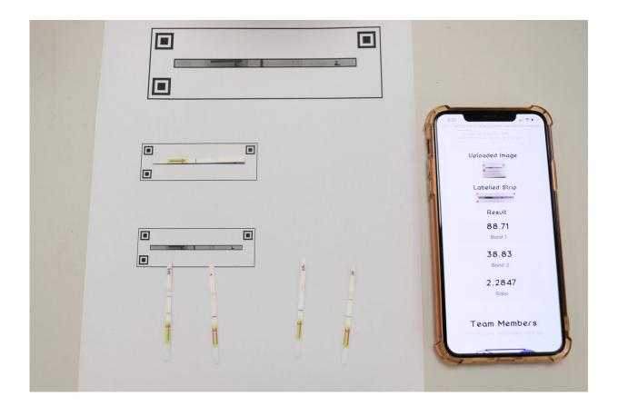
To make the test easier to use once it has been approved for roll out, the scientists integrated the test into a specially treated paper strip, and developed a mobile phone app to facilitate the interpretation of the paper strips. Credit: NTU Singapore
