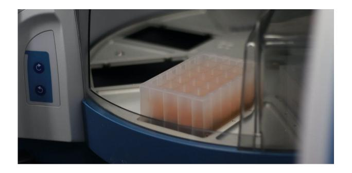
Sewage samples mixed with magnetic beads and loaded onto the liquid-handling robot for viral concentration. Credit: C. H. Sheikhzadeh @ HOMA Photographic Art
