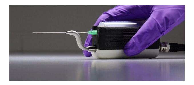
By coupling ultrasound waves to a medical needle, researchers were able to make the tip of a medical needle vibrate 30 000 times per second. The new technology could improve cancer management. Credit: Aalto University
