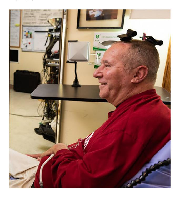
A participant in the BrainGate clinical trial uses wireless transmitters that replace the cables normally used to transmit signals from sensors inside the brain. Credit: Braingate.org
