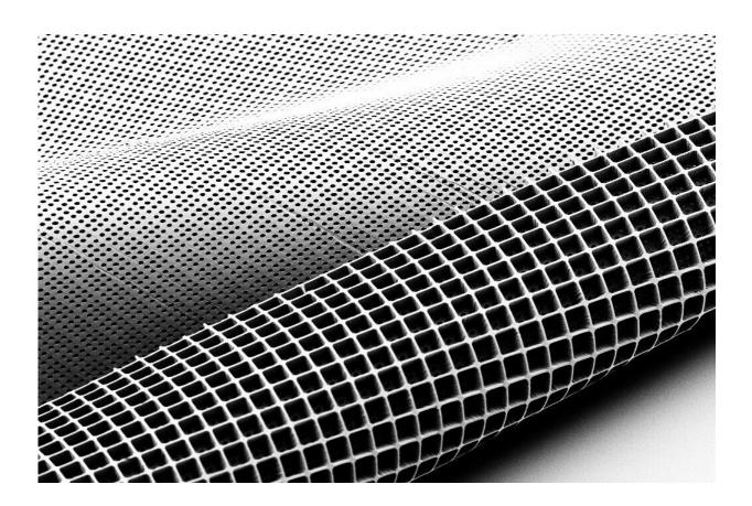
This electron microscope image of the new "scaffolding" for growing and implanting retinal cells shows the ice-cube-tray-shaped reservoirs that hold cells and cylinder-shaped holes in the bottom layer, which provide channels for maturing photoreceptors to make contact with a patient's retinal tissue. Credit: Ma Lab
