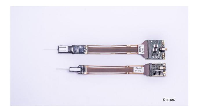
The Neuropixels 2.0 probe (bottom) is smaller than the first generation (top) and can monitor neural activity over weeks. Credit: imec
