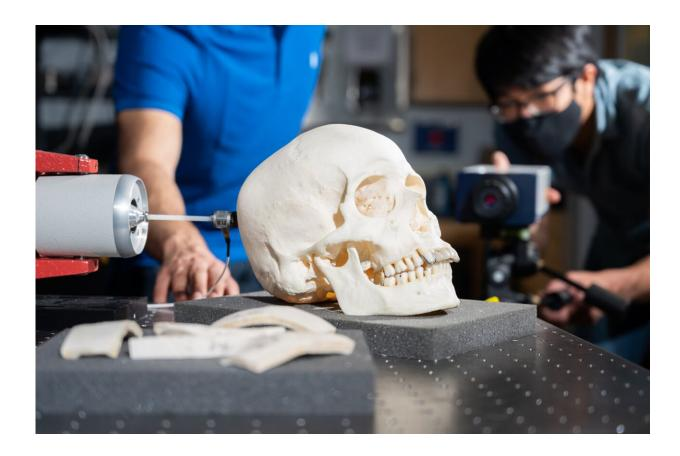
Georgia Tech researchers align the electrodynamic exciter and Laser Doppler Vibrometer setup for vibration experiments. Credit: Allison Carter, Georgia Tech
