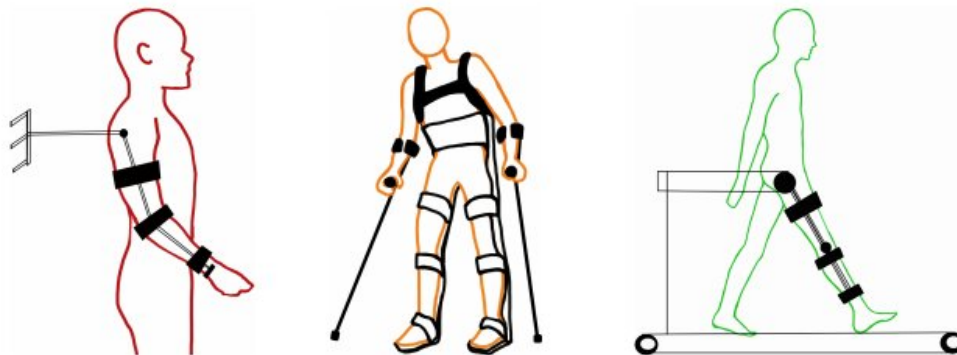
Figure 1-2: Illustration of exoskeleton devices (from left to right): upper limb exoskeleton, lower limb overground exoskeleton, lower limb body weight supported exoskeleton. Source: [3]
