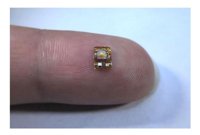
This wireless implant, developed by engineers at the University of California, Berkeley, can measure the oxygenation of living tissue deep below the surface of the skin. Credit: UC Berkeley photo by Soner Sonmezoglu
