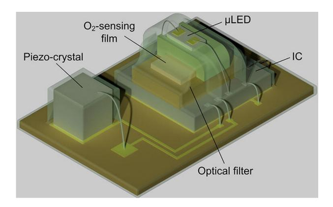
A schematic of the oxygen-detecting implant, which measures 4.5 centimeters long by 3 centimeters wide. The  $\mu$ LED, O2-sensing film, and optical filter make up the oxygen sensor, and are controlled by an integrated circuit (IC). The piezocrystal converts an electronic signal from the IC into ultrasonic waves that can be transmitted safely through living tissue. Credit: UC Berkeley image by Soner
