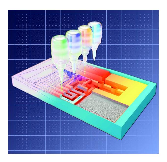
Using a 3D printer, the researchers fabricated a 3D version of a lateral flow test.
