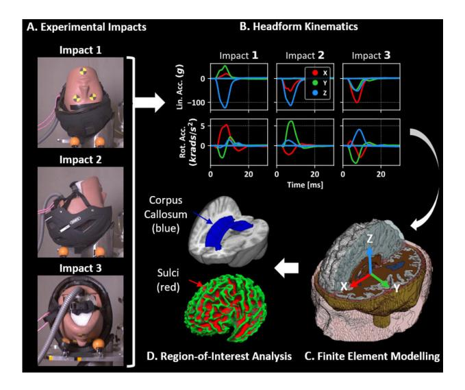
Helmeted dummy heads were dropped headfirst, side-first, and back-first onto a  $45^{\circ}$  inclined anvil. Credit: Imperial College London
