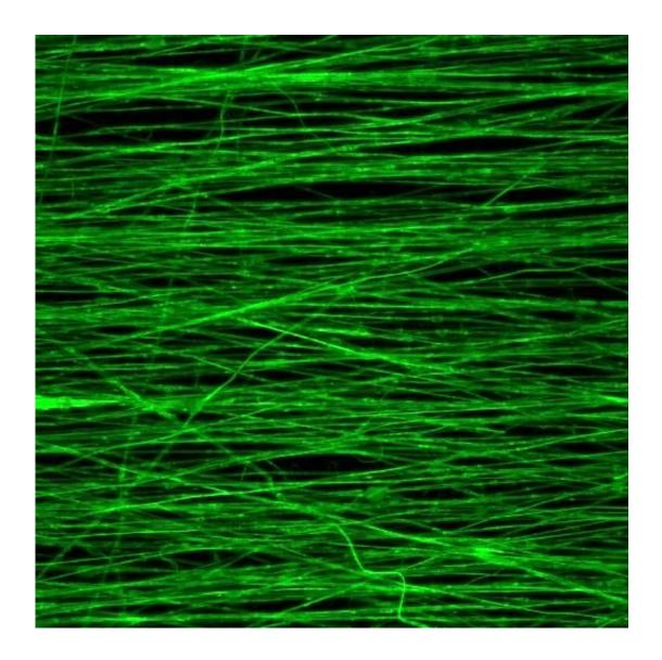
Aligned fibers produced via electrospinning can be used to form a tunable scaffold for growing new muscle, according to Rice University bioengineers. These fibers were fabricated with decellularized skeletal muscle extracellular matrix on a mandrel spinning at 3,000 rotations per minute. Credit: Mikos Research Group/Rice University
