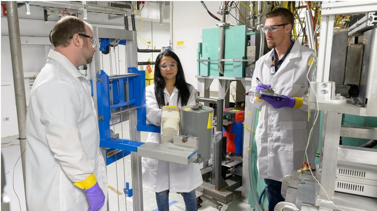
Argonne scientists prepare to load a target onto the laboratory's Low Energy Accelerator Facility, which helps to create medical isotopes. Credit: Argonne National Laboratory
