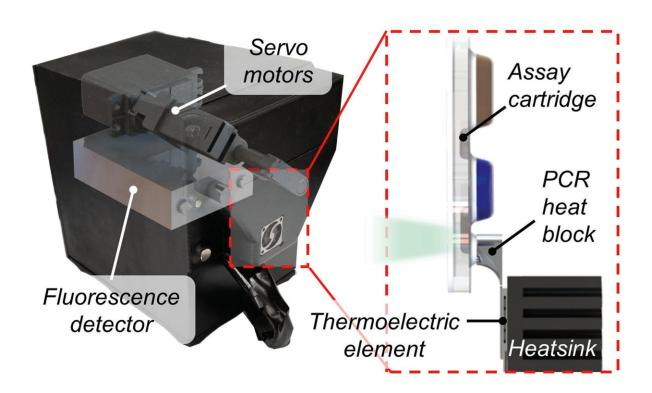
A schematic of the PROMPT instrument, showing the fluorescence detector and servo motors. Credit: A.Y. Trick et al., Science Translational Medicine (2021)
