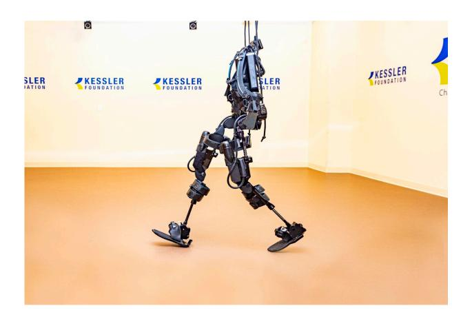
Two types of exoskeletons were used in this multi-site study, ReWalk and Ekso GT. This photo shows an Ekso GT in the Tim & Caroline Reynolds Center for Spinal Stimulation at Kessler Foundation. Credit: Kessler Foundation
