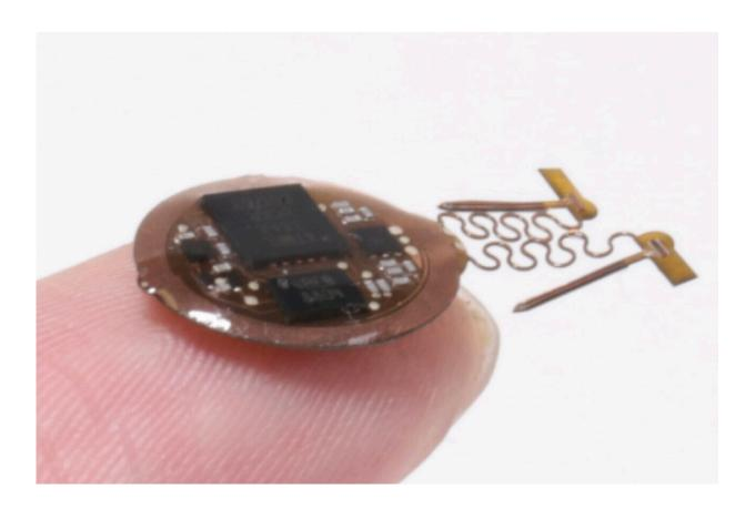
Fully implantable, wireless device enables ontogenetic research in untethered animals with dynamically programmable operation. Credit: Northwestern University
