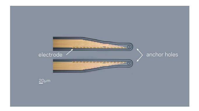
Micrograph of the micro-fabricated conformable conducting polymer-based electrode array Credit: Zifang Zhao and Claudia Cea/Columbia Engineering
