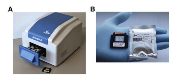
A) AriaDNA analyzer. B) Microchip for coronavirus disease 2019 detection with lyophilized reagents in the microwells displayed along with its packaging. Credit: Lumex Instruments Canada
