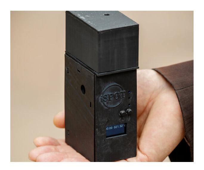
Researchers have developed a new approach to coronavirus testing, creating the first hand-held, battery-powered testing device that can yield accurate results in half an hour. The device can simultaneously test for multiple genes, researchers report. Credit: L. Brian Stauffer
