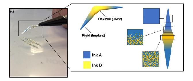
A bacteria-repelling artificial finger joint made with the new 3D print process. Credit: University of Nottingham
