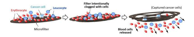
When blood flows over the microfilter, cancer cells in the blood bind to the nucleic acid aptamer. The hydrodynamic force of the blood opens the slits of the filter and the blood cells flow away, leaving the cancer cells on the filter. Credit: Associate Professor Yuta Nakashima
