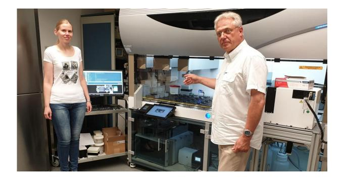
Dr. Franziska Haag (l) and PD Dr. Dietmar Krautwurst in front of the highthroughput pipetting and measuring robot (TECAN Fluent®). They use the device to investigate the odorants to which human olfactory receptors react. Credit: Leibniz-LSB@TUM
