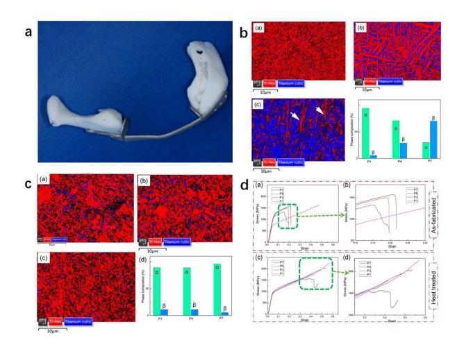
a, a typical human implant material application, which can be used as a bone plate to treat patients with transplant surgery. b, The distribution and morphology of  $\alpha$ -hcp Ti and  $\beta$ -bcc Ti in different regions of Ti-Mo samples prepared by laser solid forming (a) P1-top; (b) P4 middle; (c) P7 bottom area; (d) phase
