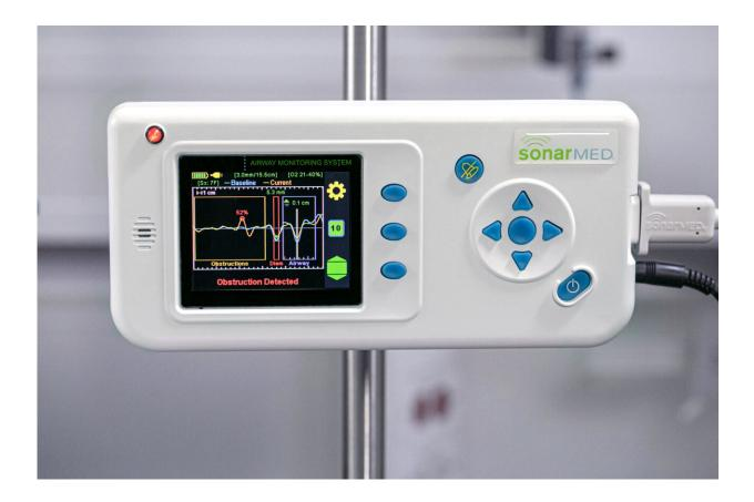
A red flashing light and audible alert from the SonarMed Airway Monitoring System help clinicians to easily see if a baby's breathing tube is obstructed or out of place. Credit: Medtronic
