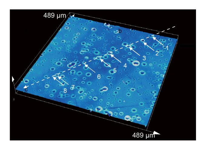
A 3D image (taken with laser confocal microscopy) shows crater-like features generated by the captured droplets. Credit: Northwestern University
