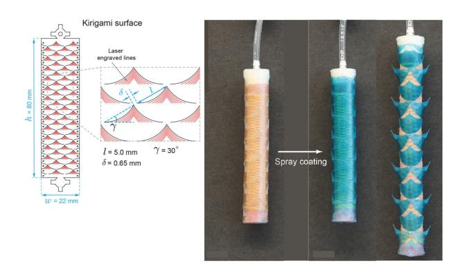
The device has two key elements -- a soft, stretchy tube made of silicone-based rubber, and a plastic coating etched with needles that pop up when the tube is stretched. Credit: MIT
