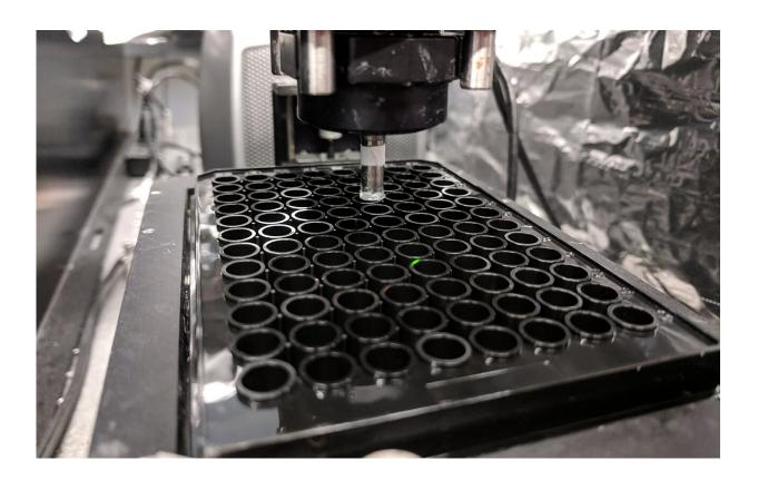
The high-throughput 3D bioprinting setup performing prints on a standard 96-well plate. Credit: Biofabrication
