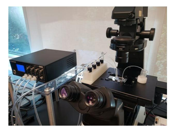
Photo of the microfluidic device on a microscope in our lab. On the left you can see the pressure pumps used to inject liquids into the chip. Credit: Elanna Stephenson
