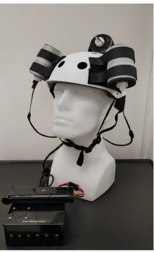
Device helmet with 3 oncoscillators securely attached. The oncoscillators are connected to a controller box powered by a rechargeable battery. Credit: Houston Methodist
