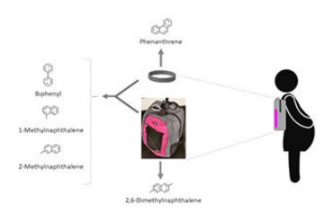
Participants in the study carried backpacks containing air-sampling equipment and a silicone wristband attached to it to analyze exposure to polycyclic aromatic hydrocarbons (PAHs). The research team found that the silicone wristbands, when used as passive samplers, have the ability to bind smaller molecular weight semi-volatile PAHs in a similar pattern as active sampling. Credit: Itza Mendoza-Sanchez
